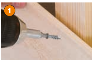
1 The variable pitch of the HECO-UNIX full thread starts to work
