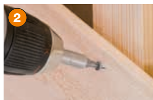
2 The smaller thread pitch means that the boards are firmly together pulled
